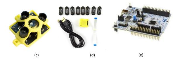
**Figure 3:** Images of parts selected (a) Pololu 12V 131:1 Metal Gear Motor, (b) Any Mark 4" Mecanum Wheel Set, (c) TeraRanger One ToF Rangefinder Type B, (d) TeraRanger Multiflex 8 Sensor Kit, (e) Nucleo STM32F446RE ARM development board,
