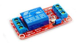
Figure 6: Picture of DZS Elec 12V Relay.
