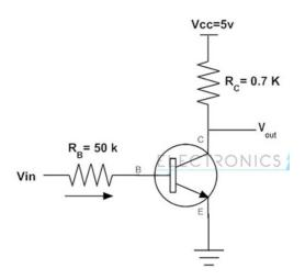
Figure 8: Circuit Connection for the Transistor.
