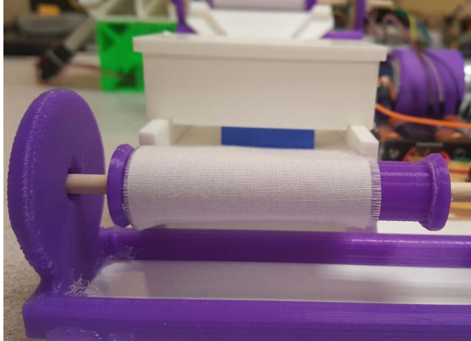
Figure 15: (b) Color Sensor Box and Conveyor Implemented
