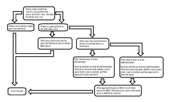
Figure 23: Grid Indexing Flowchart
