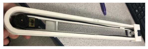
*Figure 9: Printed version of the vertical lifting pieces fitted together*
