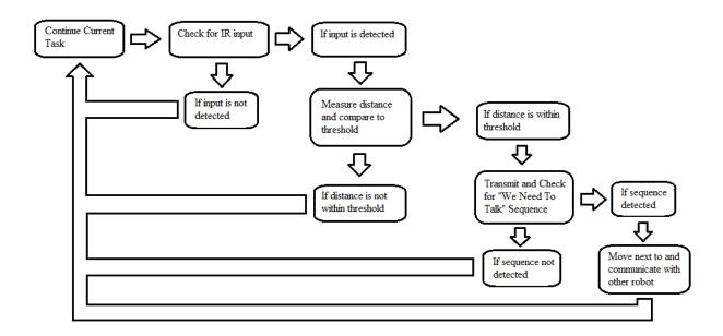
Figure 22: Communication protocol flowchart
