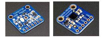
Figure 16: (a) RGB Color Sensor – TCS34725 (b) Proximity Sensor VCNL 4010
