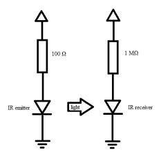
Figure 18: IR emitter and receiver circuit diagram
