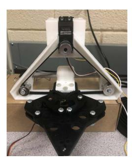
Figure 11: Printed version of horizontal lifting pieces fitted together
