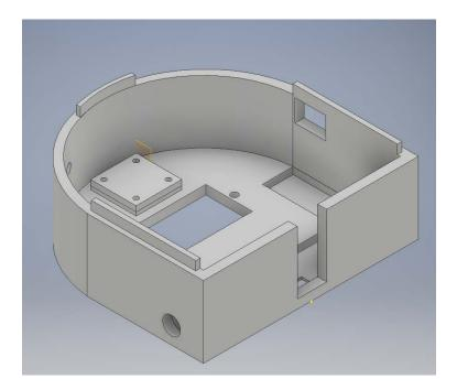
Figure 3: 3D model of the bottom of the base of the robot
