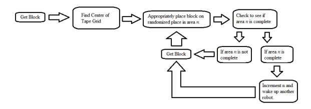
Figure 20: Block Diagram of Center Building Algorithm
