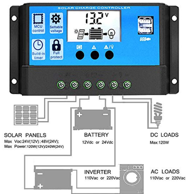
Figure 2: charge controller by PowMr. 10A 12v/24v (amazon.com)
