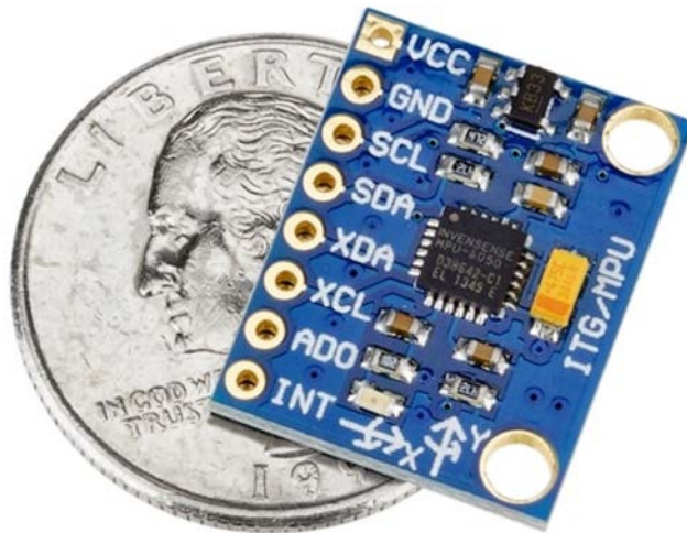
Figure B: GY-521 MPU 6050 6-Axis Accelerometer/Gyroscope
